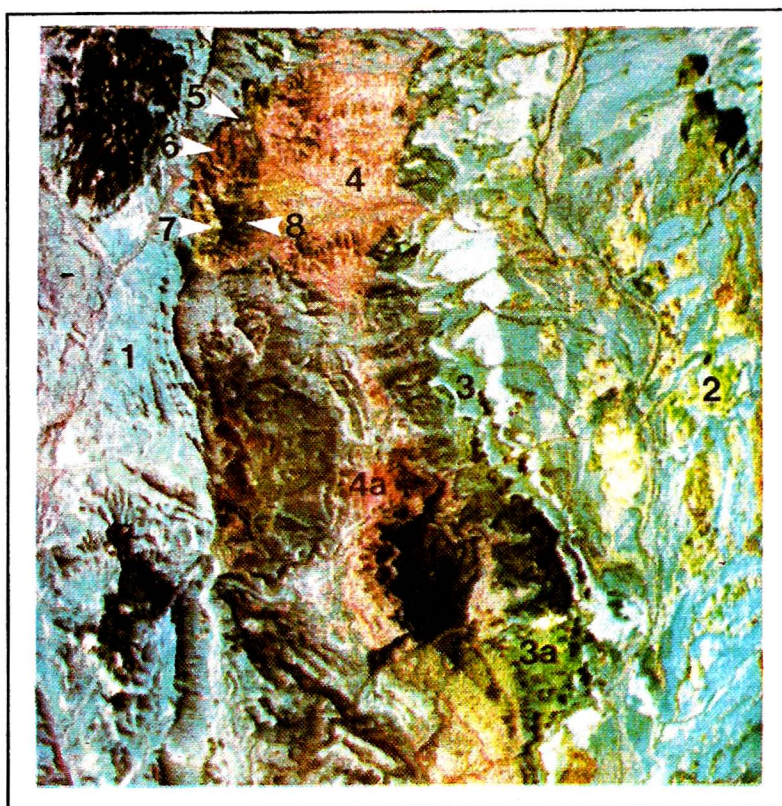
Fig. 7. Color composite of bands 48, 36 and 56, coded blue, green and red respectively. Hints to altered areas in the Shen Ramon (5-8) became visualized since solely SWIR bands are used for coding. In the composite of Fig. 6, Al-OH absorptions are masked by strong Fe- absorptions.
