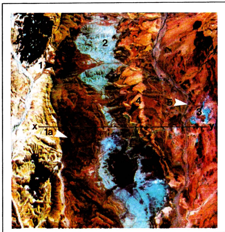
Fig. 6. Color composite of bands 1, 30 and 48, coded blue, green and red respectively. Fe-oxides appear in red due to absorptions in bands 1 and 30. Kaolinite and gypsum show cyan colors because of major absorptions in band 48. Bauxite/kaolinite are imaged green due to absorptions in the blue (1) (Fe) and red (48) (Al-OH) coded bands.
