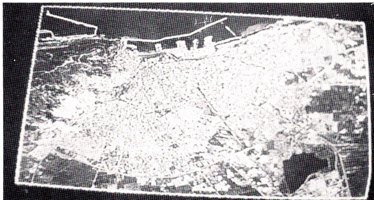
Fig. 11 - Edge detection of the rectified image with nearest neighbour resampling.
