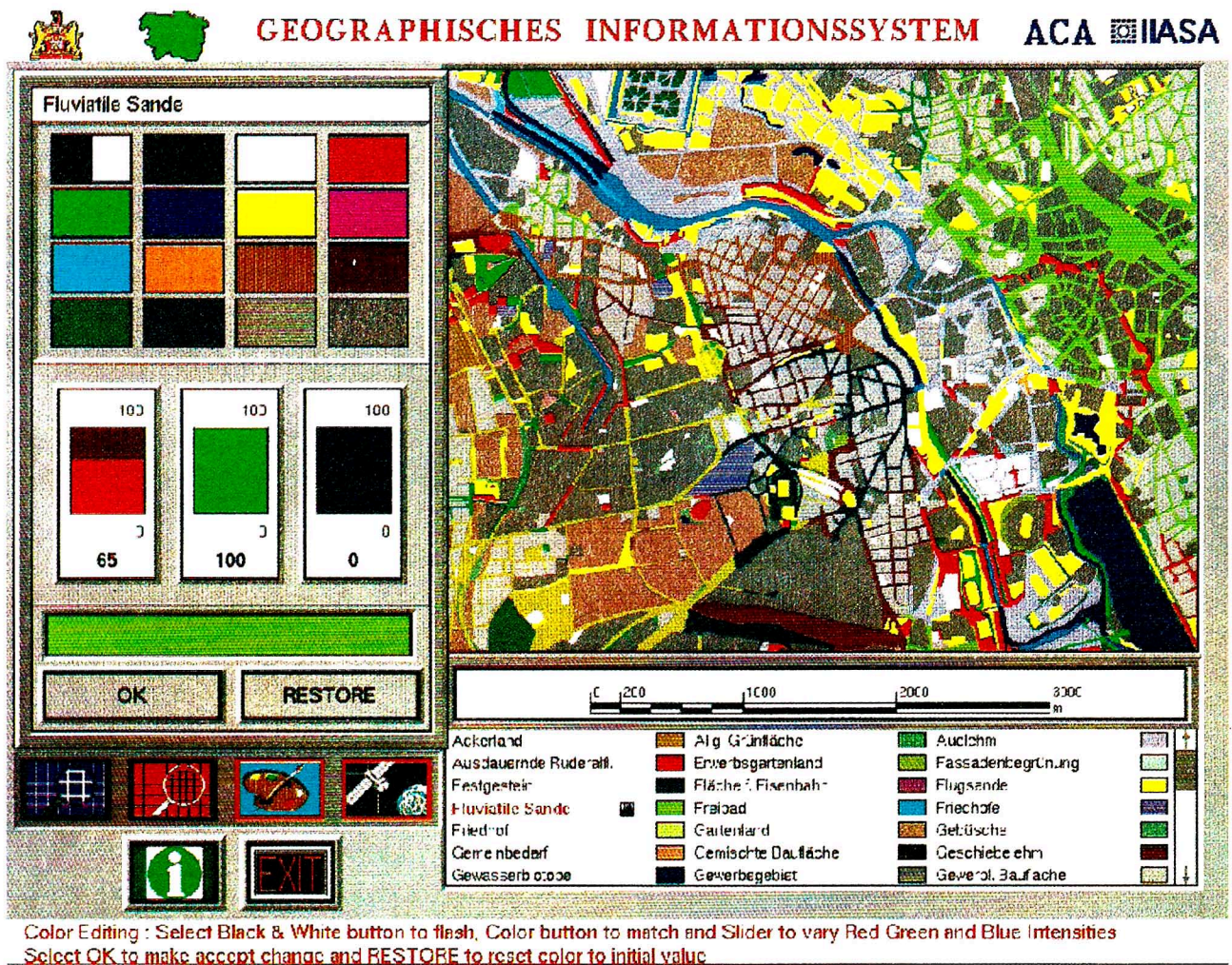
Fig. 4 - The color editor can modify individual feature display colors to design a visually attractive map for any set of features.
