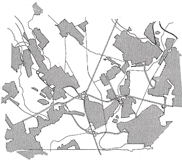
Fig. 3 - Vectorized linear objects (roads, rivers, railway routes and outlined buildup area) by photogrammetric evaluation of KFA stereo images, scale 1:100.000.
