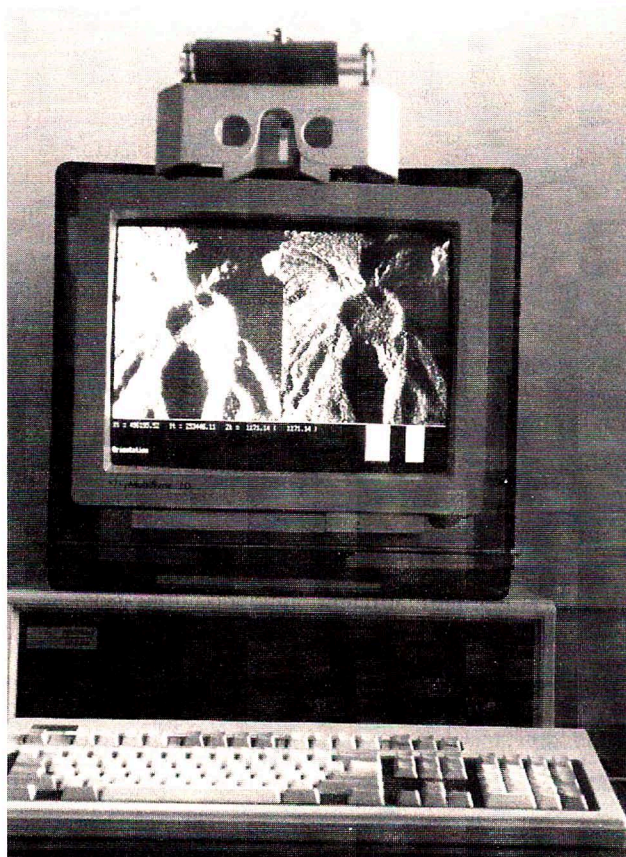
Figure 1 - The DVP System based on a Personal Computer.
