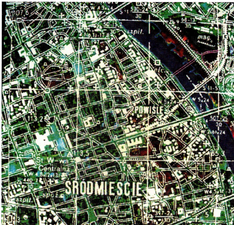
Figure 1 - Part of the satellite image map of Warsaw area reduced to the scale 1:50,000. Green areas appear red and dense built-up area in blue. Open fields are shown in white and yellow colours.
