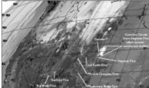
*NOAA GOES-8 Wildfire Automated Biomass Burning Algorithm (WF-ABBA) imagery, showing fires in the western US at 10:45 EDT on 9th June 2002. The WF-ABBA detects fires every half-hour over the western hemisphere*
