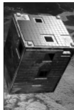
Launched in October 2001, ESA's Proba (Project for Onboard Autonomy) micro-satellite measures just 60 x 60 x 80 cm
