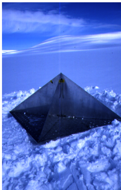
Figure 6. A radar reflector, built for the project, placed in the field in order to retrieve exact GCPs since there are very few good natural GCPs in the area.
