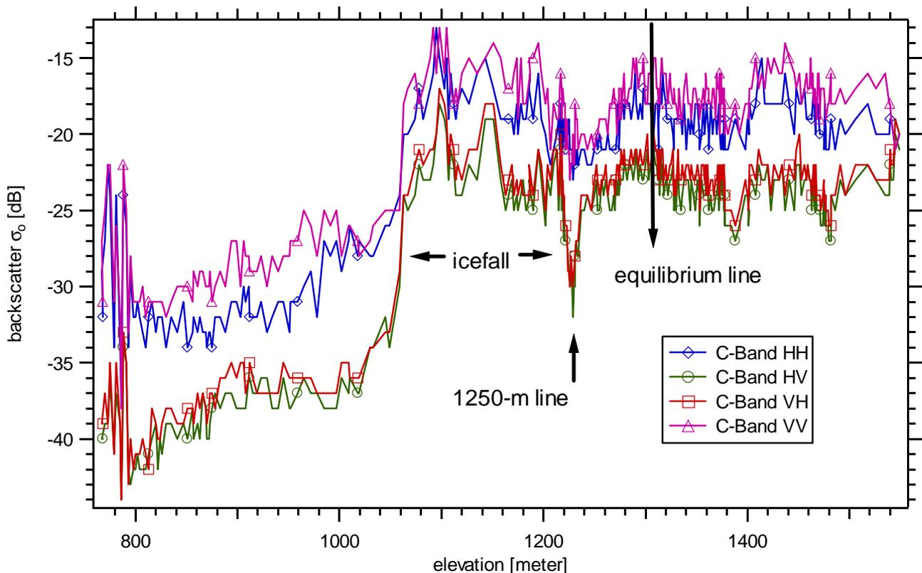
Figure 4: Backscatter along the centreline of Austre Okstindbreen for C-Band in all available polarisations. The high backscatter of the icefall can be seen between about 1050-m and 1250-m elevation. A distinct increase in backscatter at 1230-m elevation is seen in HV- and VH-polarisation, the equilibrium line, however, is located much higher at 1310 m.
