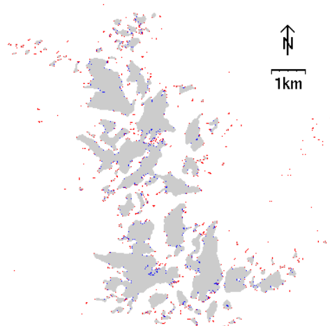
Figure 2. The influence of the 3 \times 3 median filter on the black and white glacier mask from TM 4 / TM 5 using raw DN is shown. The blue pixels were added, the red pixels deleted with the filter.
