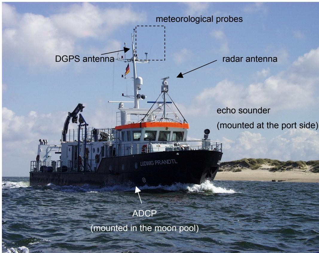
Figure 2: Measurement configuration on board Research Vessel (R.V.) Ludwig Prandtl used in the Lister Tief during the OROMA experiment on 14 August 2002.
