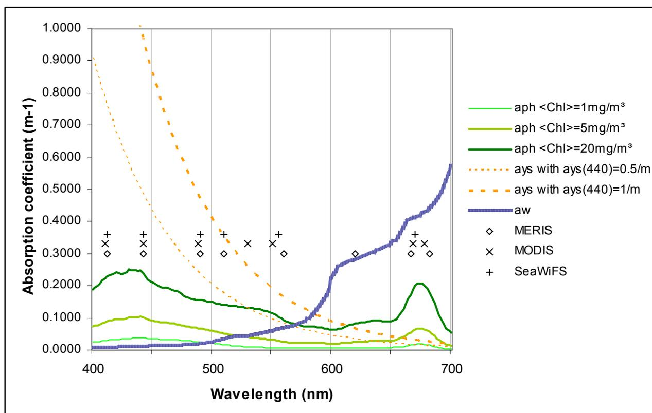
Figure 1: Absorption spectra for phytoplankton (aph) with chl *a* concentrations of 1 mg/m<sup>3</sup>, 5 mg/m<sup>3</sup> and 20 mg/m<sup>3</sup> based on (10,11), yellow substance (ays) with yellow substance absorption coefficients of 0.5 m<sup>-1</sup> and 1 m<sup>-1</sup> at 440 nm based on (12), and water (aw) based on (13). MERIS, MODIS, and SeaWiFS bands are indicated.
