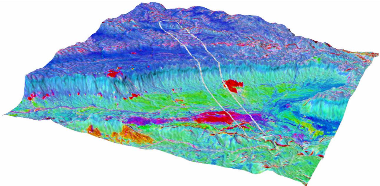
*Figure 1: Case study region Makhtesh Ramon here figured as hill shaded 3D false colour composite that is grey overlaid by the extent of the hyperspectral AISA DUAL acquisition (RGB = Landsat TM (GSD 30 m) mineral ratios 5/7 (clays), 5/4 (ferrous iron) and 3/1 (iron oxides); 3D = ASTER DEM (is a product of METI and NASA, GSD 15 m)).*
