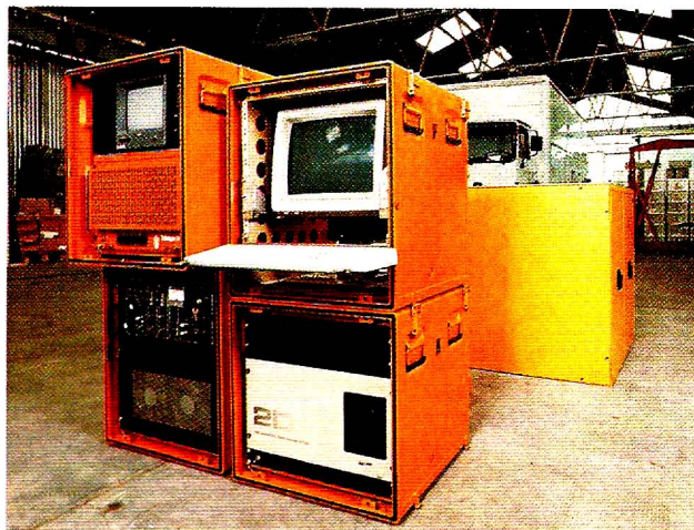
Fig. 11 - View of the TRLF, the four containers in the foreground contain the VAX computer (top left), the VAX monitor (top right), the laser power supply (bottom left) and the streak camera computer (bottom right). The larger container in the background contains the optical system.
