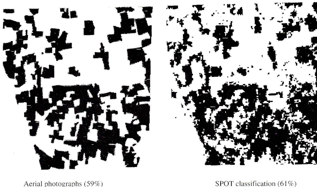
Fig. 7 - Comparison between aerial photograph interpretation and classification result for a part of the South-East region.
