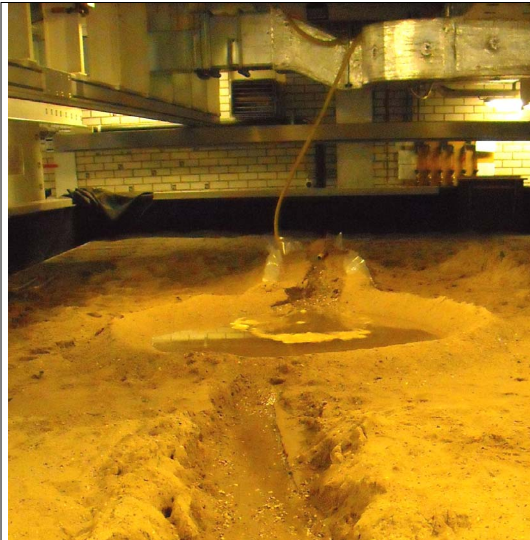
Figure 5 Experimental setup in the 'Eurotank' where we create fans and deltas within meteor craters to understand the water related processes on Mars. The centre of the photo shows a crater where a generated flow is building a delta.
