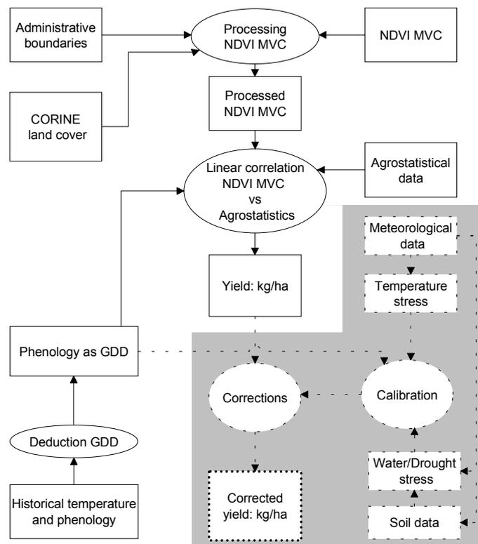
Figure 1: Schematic model for the basic (white background) and extended (grey background) NDVI linear correlation model for yield (kg ha<sup>-1</sup>).
